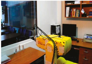
Figure 4. Fanuc LR Mate 100 iB robot. The location of the transducer on the robot arm.
