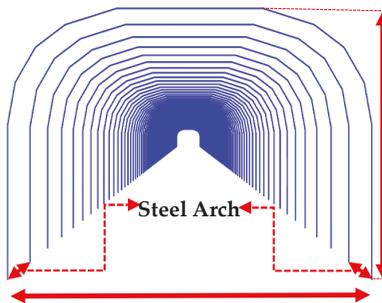
Figure 4. Modelling of steel arch for roof support.
