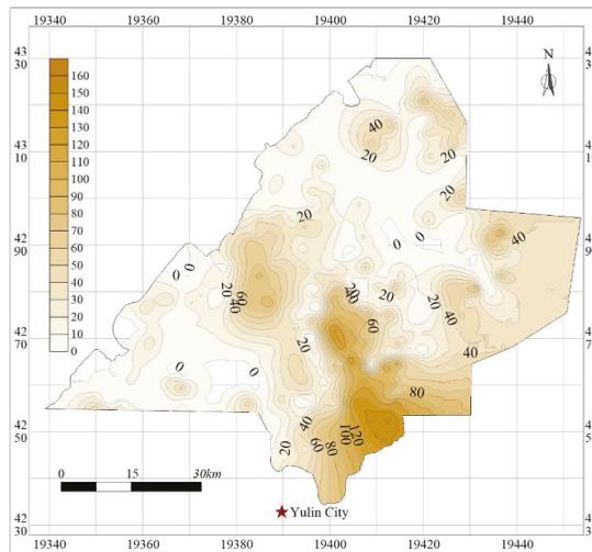
Figure 7. Aquiclude thickness contour map (Xi'an geodetic coordinate system 1980; in km).
