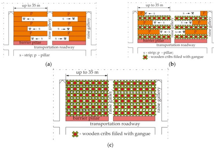
**Figure 11.** Strip mining method with the three stages of exploitation in relation to the management of wooden cribs filled with gangue: (a) First stage; (b) Second stage; (c) Third stage.
