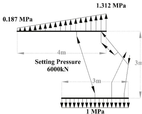
Figure 7. Pressure distribution for modeling shield support.
