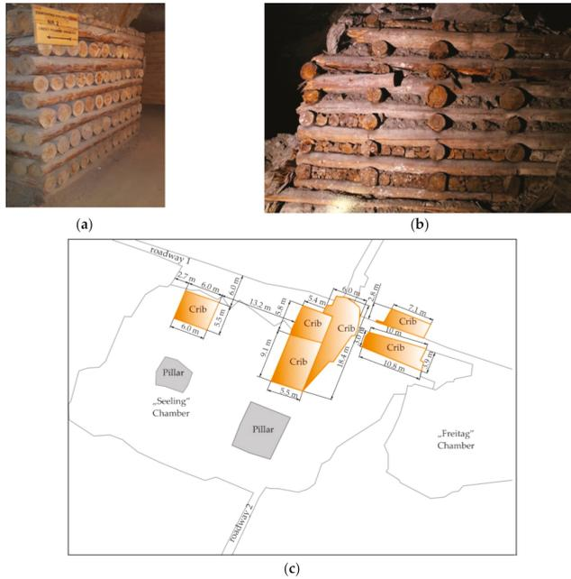
**Figure 1.** Wooden support of chamber excavations in salt mining: (a) Round wooden crib made of round beams, full in the Bochnia Salt Mine; (b) Wooden crib filled with gangue in the Wieliczka Salt Mine; (c) Protection of “Seeling” Chamber by means of wooden cribs in the Wieliczka Salt Mine.
