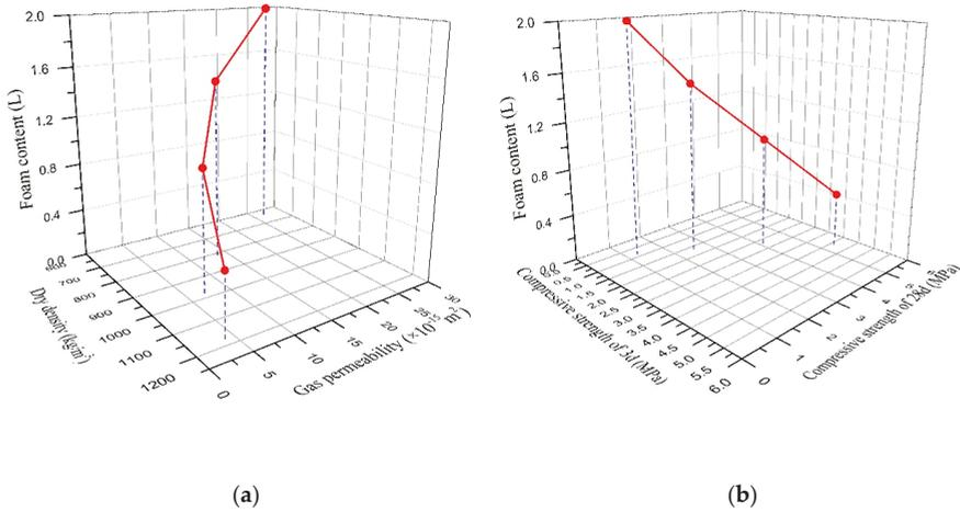
**Figure 7.** (a) The effect of foam content on dry density and gas permeability; (b) the effect of foam content on compressive strength of 3d and 28d.
