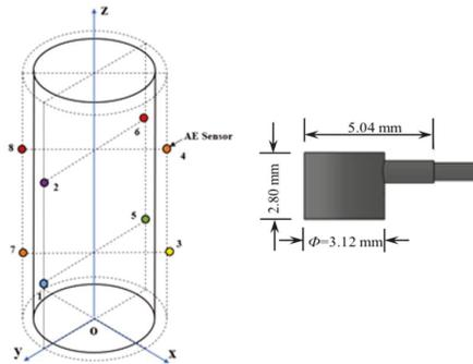
Figure 3. Distributions and dimensions of an AE sensor.
