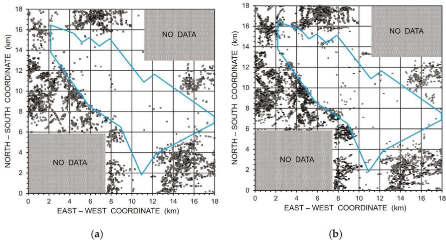
**Figure 2.** Spatial distribution of the reflectors with an additional surface movement of  $\pm 10$  mm over 10 years (grey squares), as well as the reflectors with the movement that is opposite of the global trend (plus and minus signs, respectively): (a) Period from August 1992 through August 2002; (b) period from March 2003 through March 2013.
