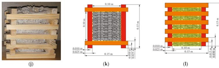
**Figure 7.** Multi-point cribs: (a) Three-point, general view; (b) Three-point, top view; (c) Three-point, side view; (d) Three-point, filled with gangue, general view; (e) Three-point, filled with gangue, top view; (f) Three-point, filled with gangue, side view; (g) Four-point, general view; (h) Four-point, top view; (i) Four-point, side view; (j) Four-point, filled with gangue, general view; (k) Four-point filled with gangues, top view; (l) Four-point, filled with gangue, side view.
