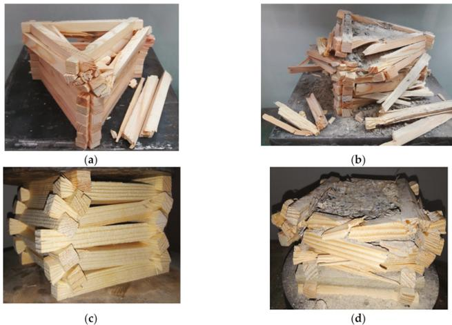
**Figure 8.** Wooden cribs models after compression test: (a) Three-point; (b) Three-point filled with gangue; (c) Four-point; (d) Four-point filled with gangue.
