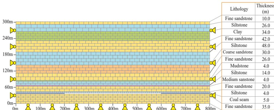
Figure 12. Numerical simulation model of sand-soil-bedrock stratigraphic structure.
