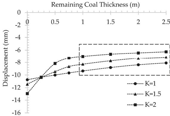
Figure 10. Correlation between roof displacements and RCT.
