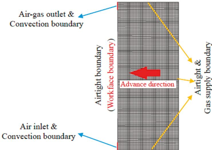
Figure 9. Computational mode and its boundary conditions.
