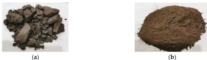
**Figure 1.** Coal gangue samples. (a) Raw coal gangue; (b) As-received coal gangue.
