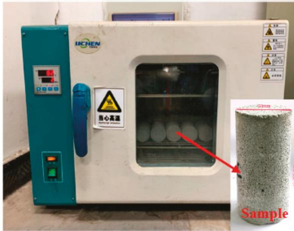
Figure 2. Constant temperature vacuum drying oven.
