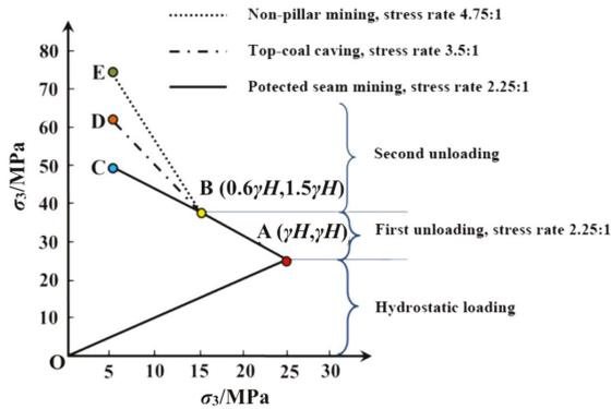
Figure 5. The loading (unloading) scheme under different mining layouts ( $\gamma H = 25 \text{ MPa}$ ).
