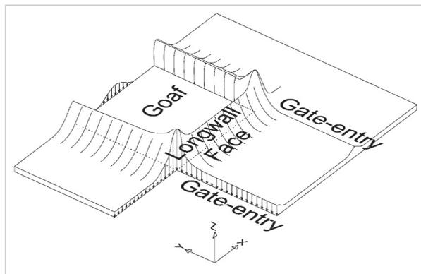
**Figure 1.** Vertical Stress Distribution during Longwall Panel Extraction.
