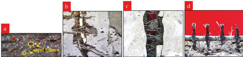
**Figure 16.** (a) Well-distributed steel fibers; bridging capacity of steel fibers in cracks: (b) P0C1S1, (c) P0C2S1; (d) fracture surface of TRM with steel fibers.
