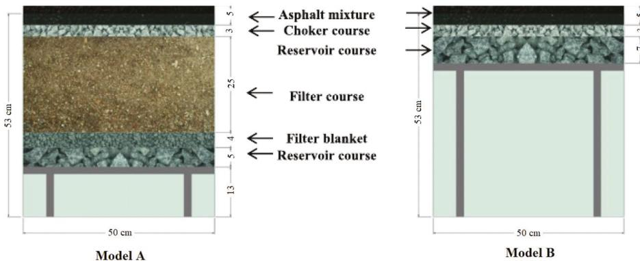
Figure 2. Permeable pavement models tested. Source: Hammes et al. [32].
