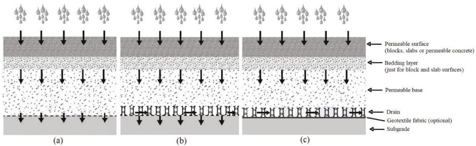
**Figure 1.** Examples of permeable pavements systems: (a) with total infiltration; (b) with partial infiltration; (c) without infiltration. **Source:** Based on ABNT [17].
