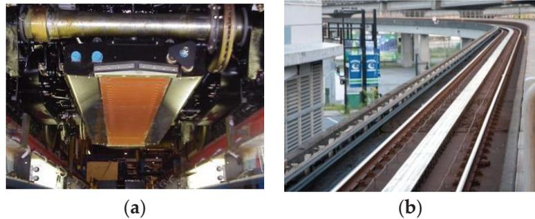
**Figure 3.** LIM primary (supplied part) (a); LIM secondary (reaction rail) (b) [28].
