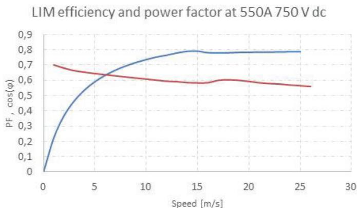
**Figure 16.** Power factor and efficiency curves for one example of a traction LIM.
