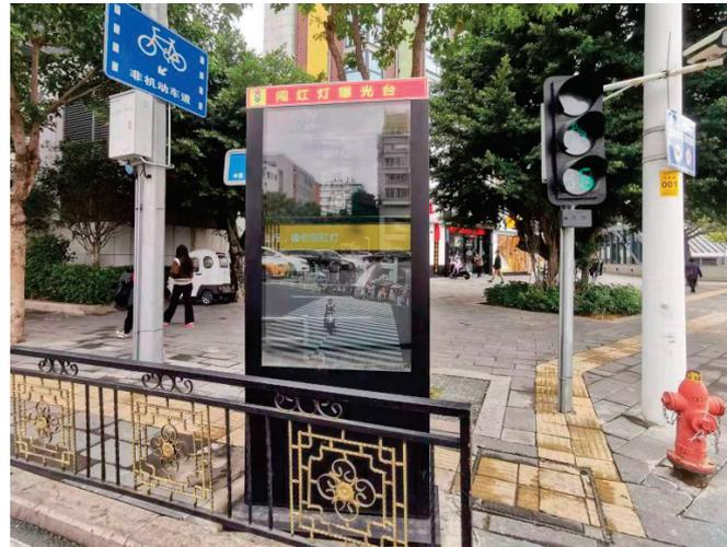
Figure 2. Part of the red-light monitoring system.
