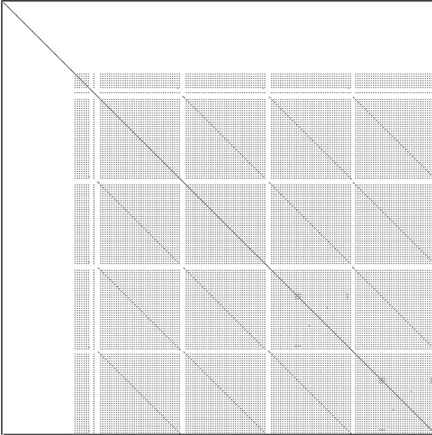
Figure 8.5: Dotplots produced by four switch statements.
