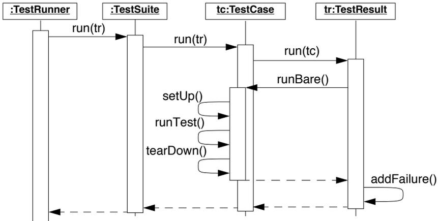
Figure 6.5: In JUnit, tests are actually run by an instance of `TestResult`, which invokes the `runBare` template method of a `TestCase`. The user only needs to provide the `setUp()` and `tearDown()` methods, and the test method to be invoked by `runTest()`.
