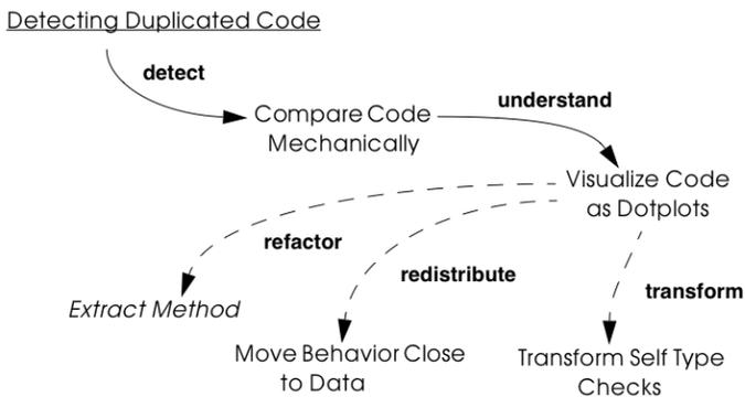
Figure 8.1: Two patterns to support Detecting Duplicated Code.
