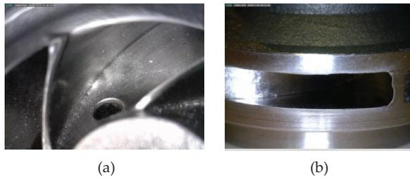
**Figure 10.** Details of Impeller 2 (after media change) showing (a) interior surface and (b) pressure side.
