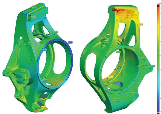
**Figure 7.** Dimensional changes of printed model (PMMA–BJ method).
