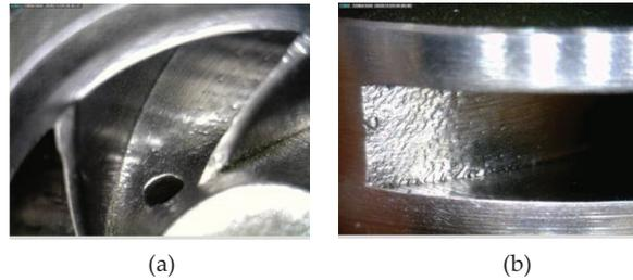
**Figure 9.** Details of first impeller (after tooling optimization) showing (a) interior surface and (b) pressure side.
