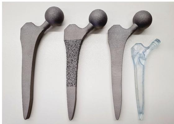
**Figure 5.** The successfully manufactured solid (left), porous (middle) and selectively hollowed (right) hip implants. The solid and selectively hollowed implants look identical. Thus, a clear resin plastic version of the selectively hollowed implant is also shown to indicate the internal structure of the selectively hollowed implant (right).
