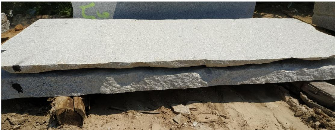
Figure 3. Offcuts (2.5 m long, 1.5 m wide, 0–0.1 m thick).
