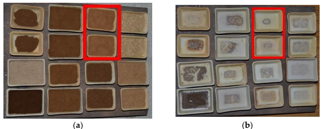
**Figure 2.** Miscanthus after wet torrefaction in different process conditions (samples after wet torrefaction in 200 °C, 10 min, water: biomass ratio 12:1): (a) raw samples; (b) samples after 3 h of ashing in the furnace at 850 °C.
