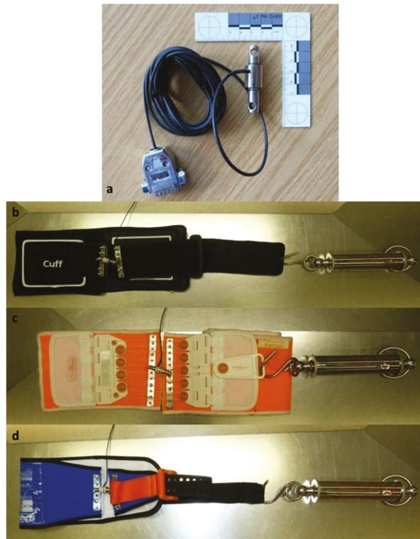
**Figure 1.** Used devices: (a) Newtonmeter; (b) Pneumatic pelvic sling VBM<sup>®</sup> prepared with Newtonmeter and tension spring; (c) T-POD<sup>®</sup> prepared with Newtonmeter and tension spring; (d) SAM Sling<sup>®</sup> prepared with Newtonmeter and tension spring (source: Haussmann [22], modified).
