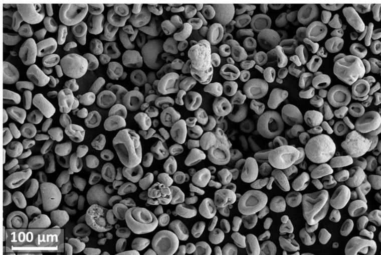
Figure 4. SEM image of W-C-Co microgranules obtained in the process of spray drying.
