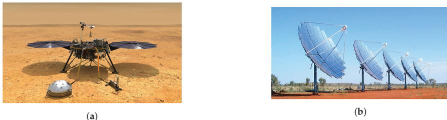
**Figure 1.** Some examples of solar cells use in space and terrestrial applications: (a) NASA's InSight Lander robot, powered by solar energy, and already owns the off-world record of power generation. (b) A HCPV parabolic system that uses high-efficiency multi-junction modules by Solartron Energy Systems.
