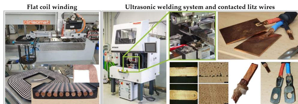
**Figure 5.** Manufacturing cell for flat coil winding (left), ultrasonic welding system and contacted litz wires (right).
