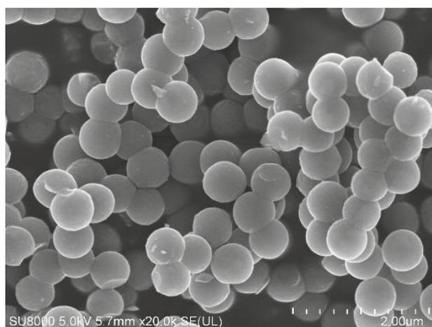
Figure 2. SEM image of the used carbon spheres.
