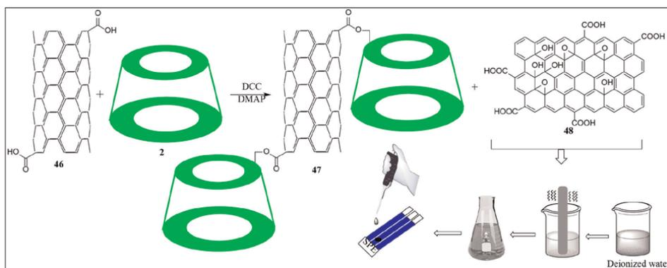
**Figure 12.** Schematic illustration for the development of bisphenol A electrochemical sensor via modification of SPE with  $\beta$ -CD and graphene oxide-functionalized MWCNTs.
