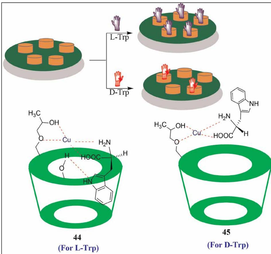
**Figure 11.** Schematic illustration of electrochemical recognition of the chiral enantiomers of tryptophan (Trp) via hydroxypropyl  $\beta$ -CD-based electrochemical sensor.
