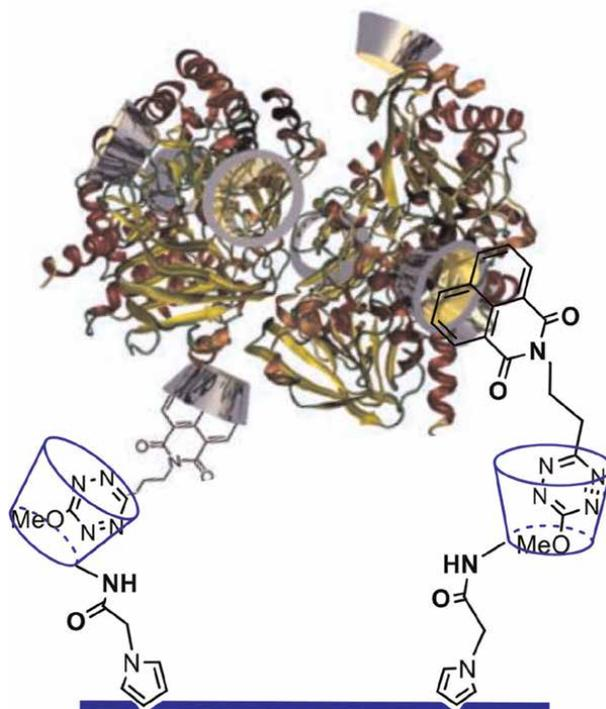
**Figure 19.** ITO electrode covered by assembly containing glucose and naphthalimide fragment.
