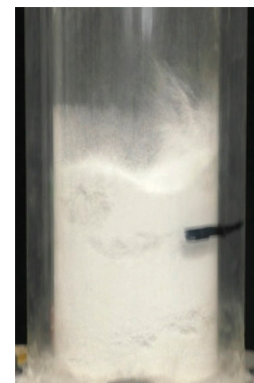
Figure 8. Classification of flow pattern and snapshots of \text{Al}_2\text{O}_3 by vertical vibrating fluidization. (a) Classification of flow pattern. (b) Fluidization bed (Region III). (c) Dispersion bed (Region IV).
