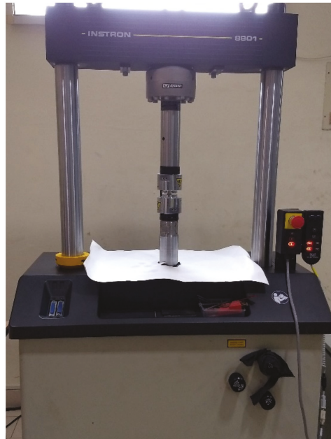
Figure 8. Instron 8801 UTM for tensile and bending test.
