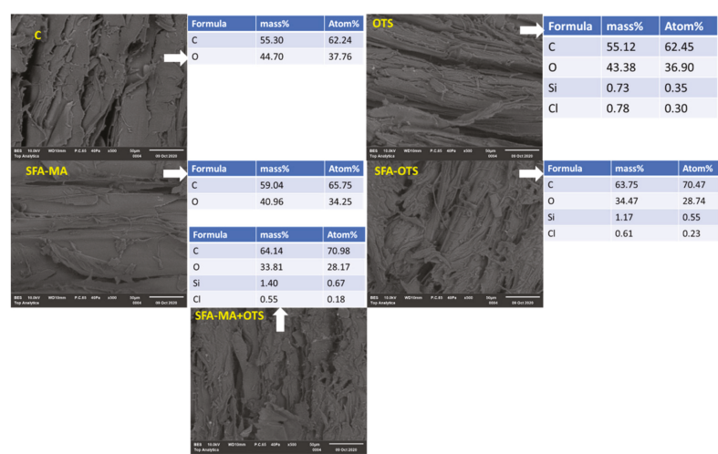
Figure 4. SEM-EDS analysis of aspen wood coated with hydrolysate-based coatings and an uncoated reference wood (sample C). The SEM micrographs were captured at a scale of 100 \mu\text{m} . The EDS scanning was performed at the same scale and surface.
