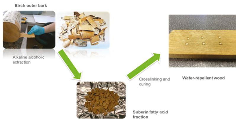
Figure 1. Schematic of SFA extraction and hydrophobic coating on wood.
