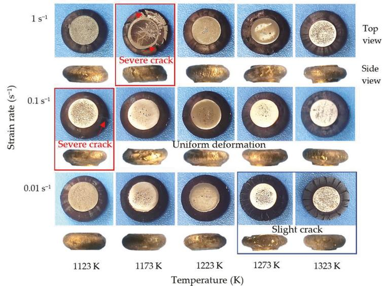
Figure 2. Macro-appearance (top and side views) of deformed alloys at different processing conditions.
