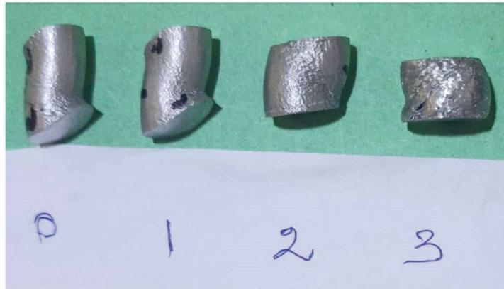
Figure 17. Distorted compression test specimens.
