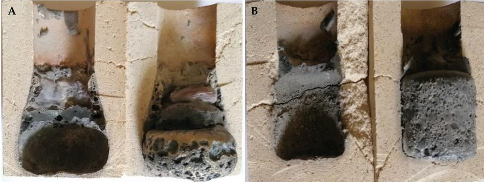
**Figure 7.** Degradation of refractory material F 36 after high-temperature testing; (A) steel XT 720, (B) steel 11 523.
