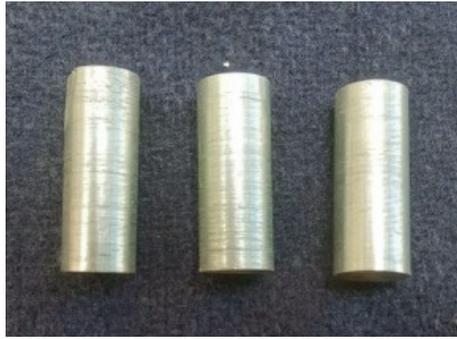
Figure 3. Compressive test specimens.
