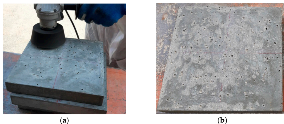
Figure 8. (a) Process of polishing the casting surface; (b) Surface after polishing.
