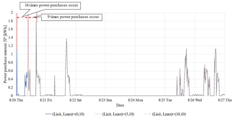
Figure 13. Changes in the power purchase amount at  $L_{max} = 10$  [kWh] and  $L_{init} = 0, 5, 10$  [kWh].
