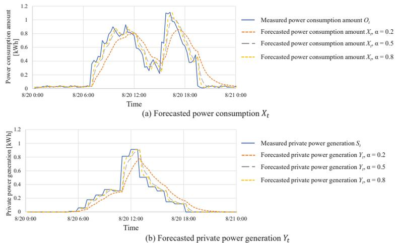
**Figure 8.** Predicted vs. measured power consumption amount  $X_{t+1}$  power generation  $Y_{t+1}$  based on  $\alpha$  values of 0.2, 0.5, and 0.8.
