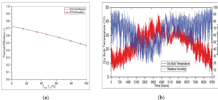
**Figure 7.** (a) Comparison of collector efficiency curve (simulation vs. experimental data reported by the collector’s manufacturer at  $G = 1000 \text{ W/m}^2$ ); (b) daily temperature and humidity variation for Lahore, Pakistan.
