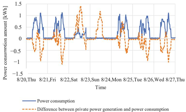
**Figure 11.** Power consumption and difference between private power generation and power consumption.
