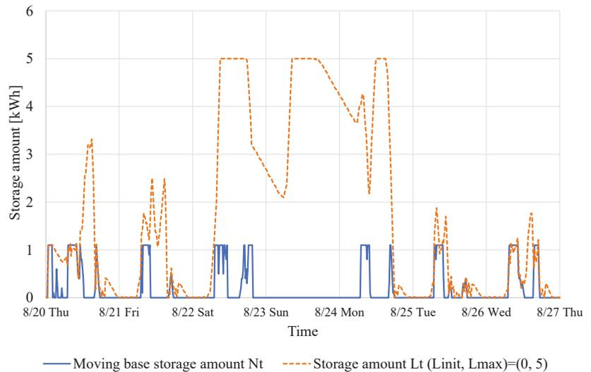
**Figure 9.** Moving base storage amount  $N_t$  and storage amount  $L_t$  ( $L_{init} = 0$  kWh,  $L_{max} = 5$  kWh) over the period analyzed.
