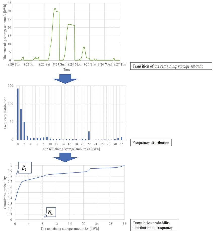
**Figure 5.** The calculation procedure for the cumulative probability distribution  $F(L_t)$  with the remaining storage capacity  $L_t$  and the moving base inventory  $N_t$ .
