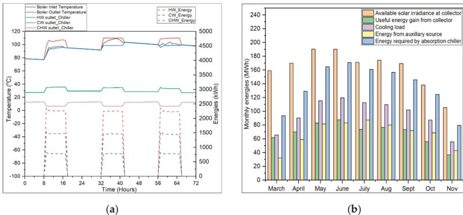
**Figure 10.** (a) Chiller outlet temperature and energies of hot water, cooling water and chilled water loop for three days from 03.06. to 05.06. (b) evacuated tube collector (ETC) + absorption chiller results at collector area ( $A_c$ ) = 1000 m<sup>2</sup>.
