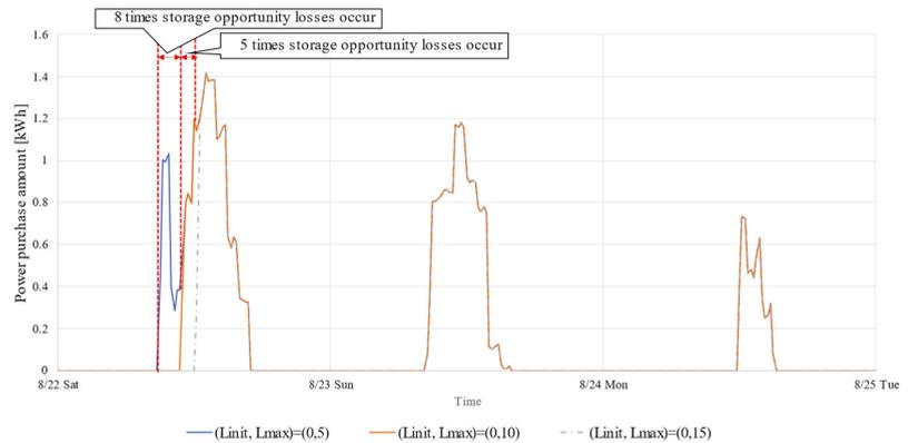
**Figure 15.** Changes in the power purchase amount when the initial inventory amount  $L_{init} = 0$  [kWh] and the maximum storage capacity  $L_{max} = 0, 5, 10$  [kWh].
