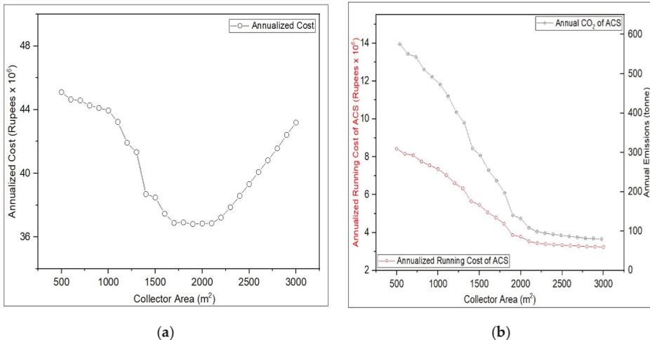
**Figure 12.** (a) Variation of annualized cost of ACS by varying collector area; (b) variation of annualized running cost and annual CO<sub>2</sub> emissions of ACS by varying collector area.
