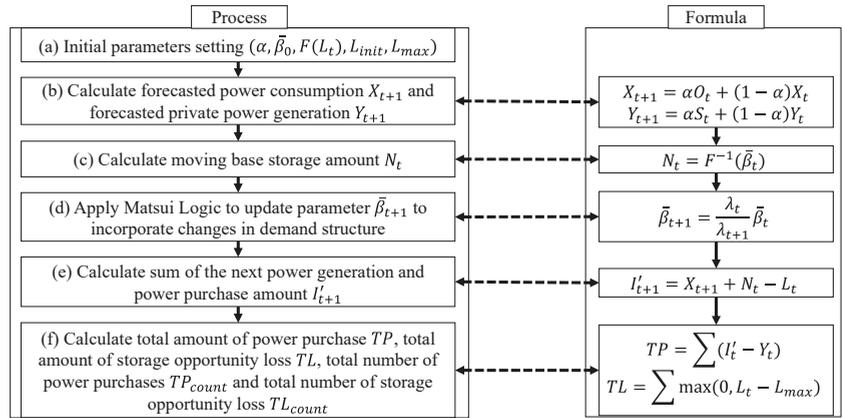
Figure 4. Procedure for applying the on-demand DSMM to renewable power generation.
