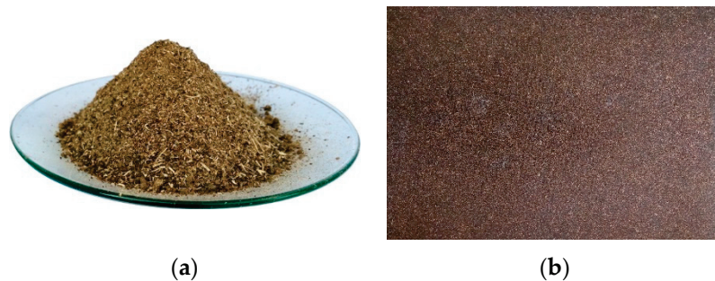
Figure 3. (a) Dry-compounded feedstock and (b) sample board, after hot-pressing at 180\text{ }^{\circ}\text{C} for 30 min.
