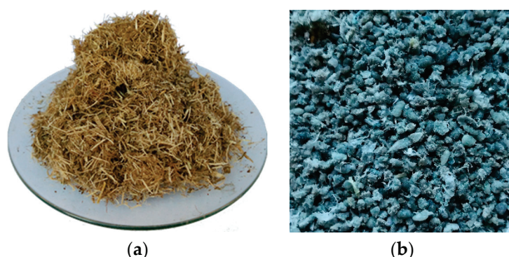
Figure 1. (a) Milled whole-tree biomass of A. saligna and (b) rLDPE.
