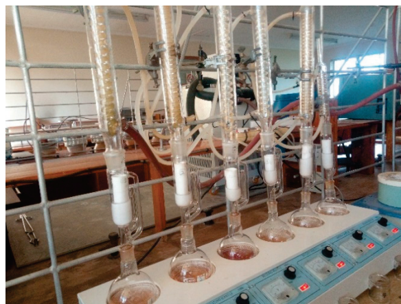
Figure 5. Soxhlet extraction setup for biomass compositional analysis.
