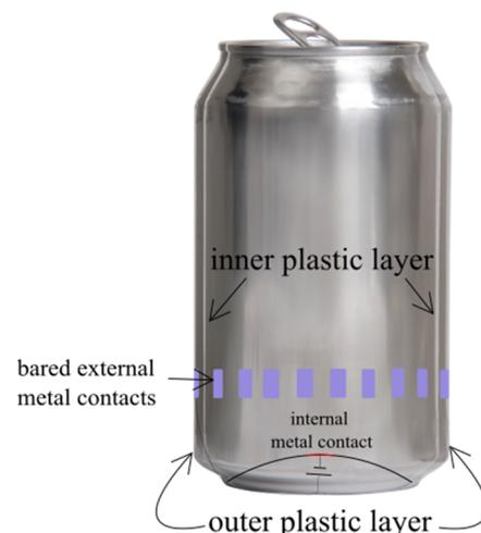
**Figure 6.** Structure for salt-based taste altering soda.
