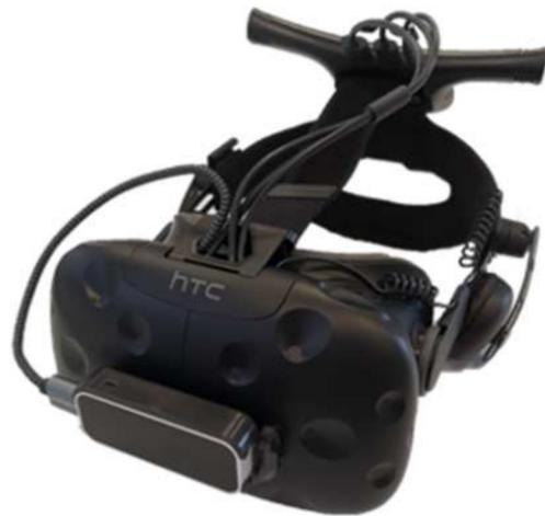
**Figure 1.** HTC VIVE glasses with Leap Motion.
