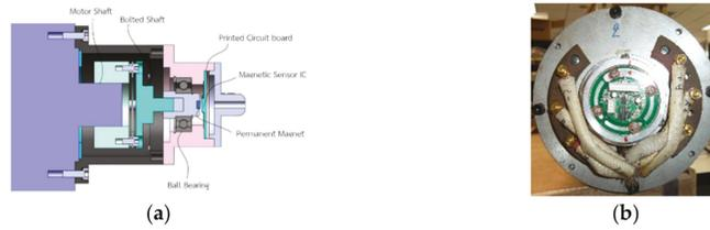
**Figure 16.** Rotor position detection system: (a) mechanical coupling device; (b) a constructed rotor position detection system installed on the three-phase 6/4 pole SRM.
