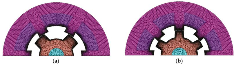
Figure 5. Mesh size of FEA model (a) 6/4 SRM; (b) 8/6 SRM.
