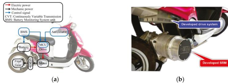
**Figure 1.** The electric motorcycle driven by the SRM and drive system. (a) The schematic of the electric motorcycle system; (b) the installed SRM and drive system.
