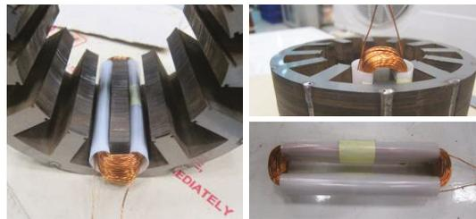
Figure 11. One coil winding on the stator pole.
