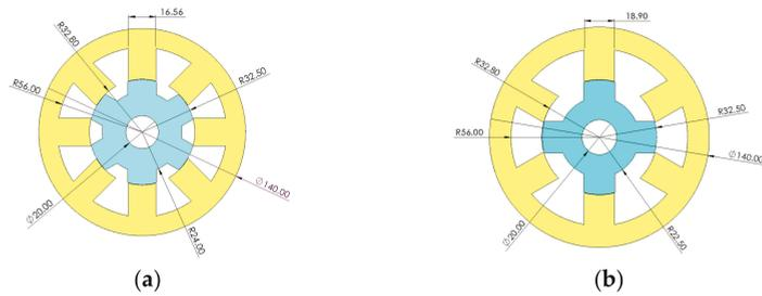
**Figure 3.** Outline of the designed motor: (a) four-phase 8/6 pole SRM; (b) three-phase 6/4 pole SRM.
