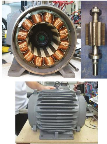
**Figure 13.** Stator, rotor, and completed 12/8 SRM prototype.
