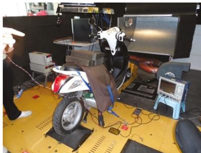
**Figure 19.** Test run of the constructed electric motorcycle on a chassis dynamometer.
