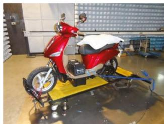
Figure 22. EMI/EMC testing of the constructed electric motorcycle.
