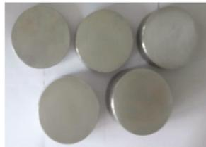
**Figure 6.** Aluminum specimens after surface machining.
