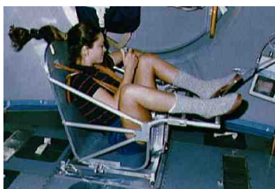
h / Astronaut Tamara Jernigan measures her mass aboard the Space Shuttle. She is strapped into a chair attached to a spring, like the mass in figure g. (NASA)
