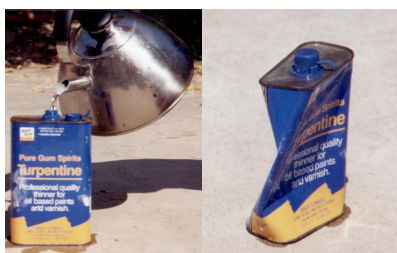
a / A vivid demonstration that heat is a form of motion. A small amount of boiling water is poured into the empty can, which rapidly fills up with hot steam. The can is then sealed tightly, and soon crumples.
