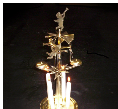
b / A heat engine. Hot air from the candles rises through the fan blades, and makes the angels spin.
