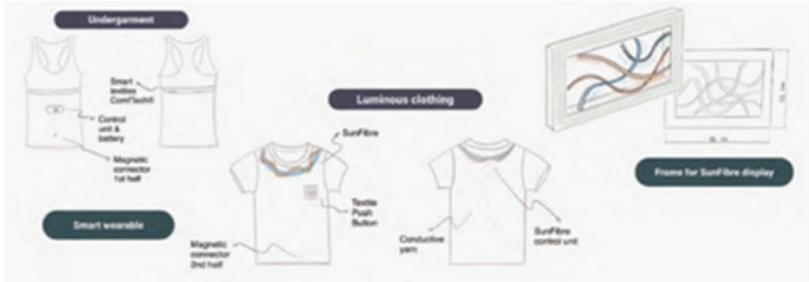
*A smart garment that monitors stress level, thanks to Smart textiles ComTech. Through the use of SunFibre, a lighting tech, it displays the mood of the person wearing it, calling others to action.*
