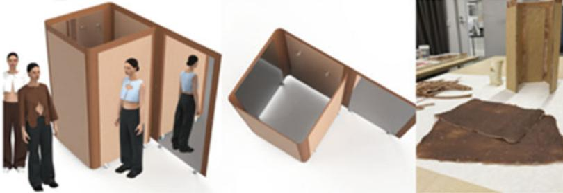
*We aimed to create a flexible mobile fitting room that could be used in flea markets that are short on space using sustainable bio-based materials.*
