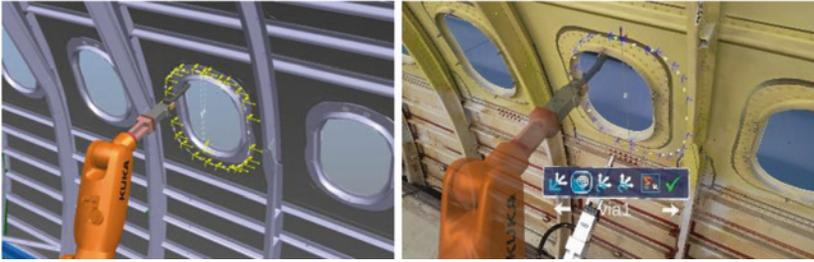
**Fig. 7** Program in simulation system (left); Displaced program in reality (right)
