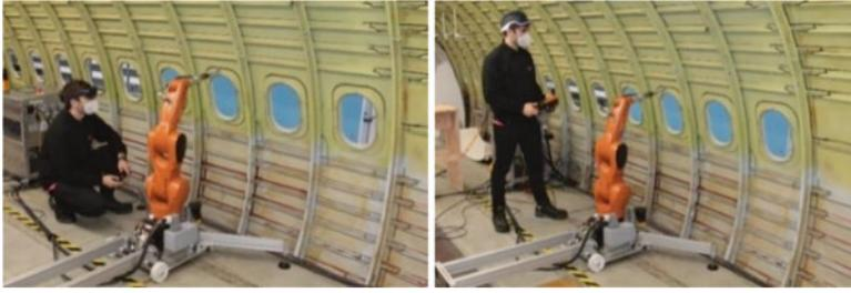
**Fig. 5** User during programming with AR (left) and Teach-In (right)
