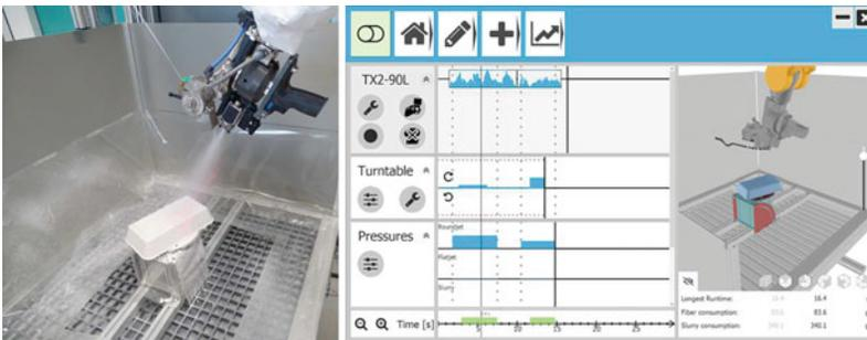
**Fig. 1** Given a setup with a turntable and workpiece (left), our goal is to know this setup in the 3D simulation of our programming framework (right)
