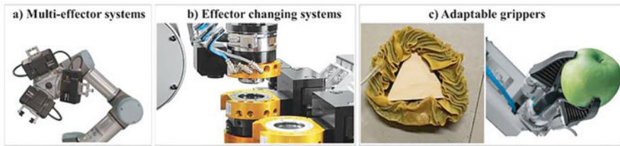
**Fig. 1** Solutions for gripping different objects [6–9]
