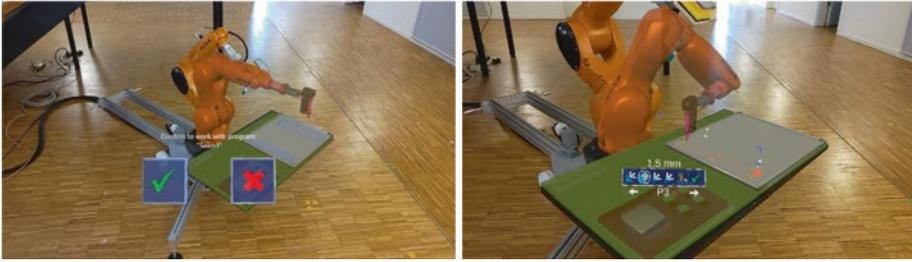
**Fig. 2** AR view of the MiReP system prior and post program optimisation
