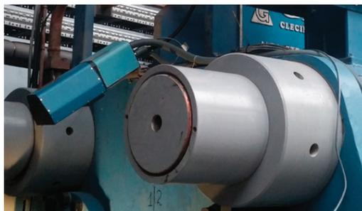
Figure 4. Pyrometers' positions.
