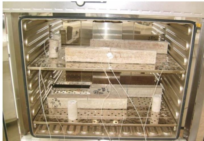
**Figure 4.** Temperatures control through installation of thermocouples.
