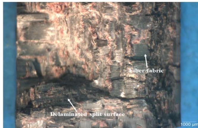
**Figure 23.** Typical optical macrograph of a specimen of HRJ-15881-based CFRP composite modified with 0.5 wt.% SiC tested at 28 kg m/s.
