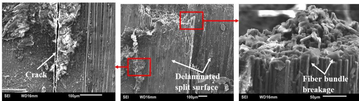
**Figure 27.** Typical SEM fractographs of HRJ-15881-based CFRP composites modified with 2 wt.% CS after SHPB testing at 28 kg m/s.
