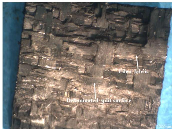
**Figure 24.** Typical optical macrograph a specimen of HRJ-15881-based CFRP composite modified with 2 wt.% CS tested at 28 kg m/s.
