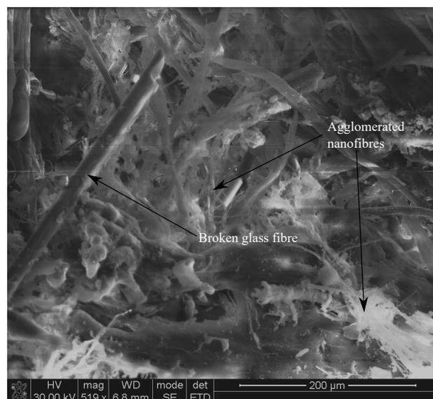
**Figure 8.** Agglomerated nanofibers of 1 wt% RONFs mats strengthened hybrid composite.
