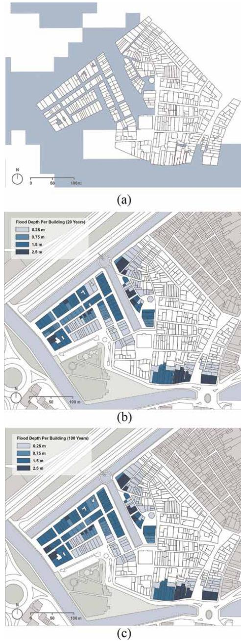
**Figure 10.** Hazard levels: (a) flood depth hazard map for 100 years return period; (b) flood depth per building for 20 years return period; (c) flood depth per building for 100 years return period.
