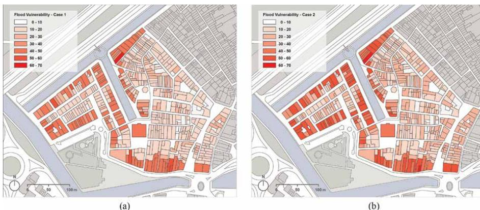
**Figure 8.** Flood vulnerability index results: Distribution over the study area Case 1 (a) and Case 2 (b).
