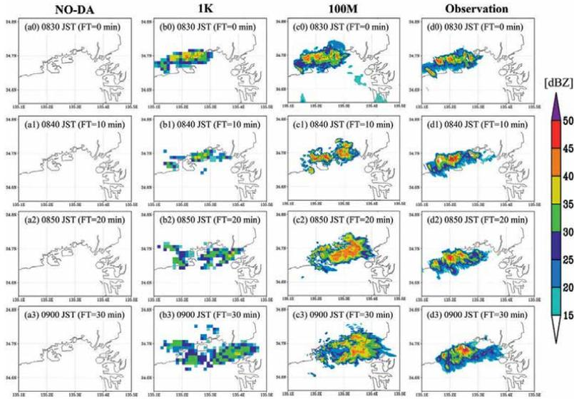
**Figure 7.** Radar reflectivity [dBZ] at 2-km elevation for (a0–a3) NO-DA, (b0–b3) 1 K, (c0–c3) 100 M and (d0–d3) PAWR observation. Top, second, third and bottom rows correspond to 0830 (initial time), 0840 (10-minute forecast), 0850 (20-minute forecast), 0900 JST (30-minute forecast), respectively.
