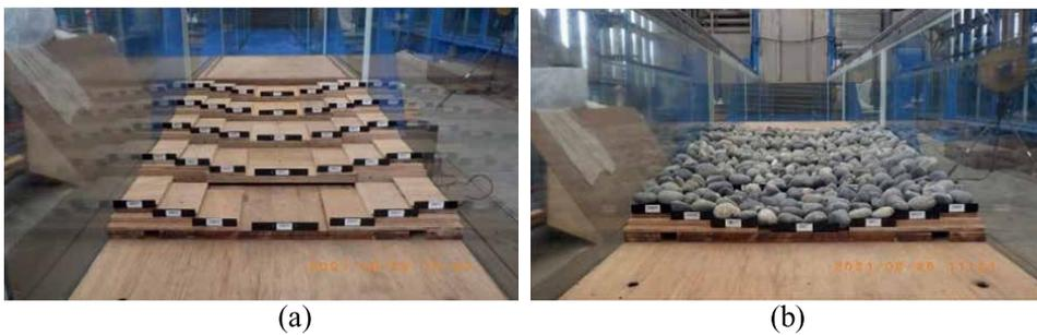
**Figure 5.** Symmetric model of consecutively assembled boulders (1/12.5 slope). (a) Stepped channel as a base. (b) Consecutively assembled boulders.
