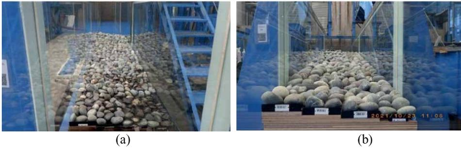
**Figure 4.** Half model of consecutively assembled boulders. (a) Half model with 1/25 slope. (b) Half model with 1/8.5 slope.
