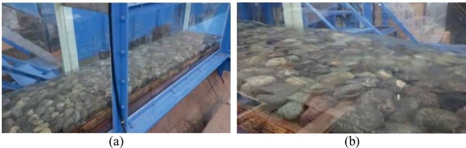
**Figure 6.** Flow conditions for a  $1/25$  downward slope and a transverse slope around  $1/8$ . (a) Flow condition for Case 4. (b) Flow condition for Case 2.
