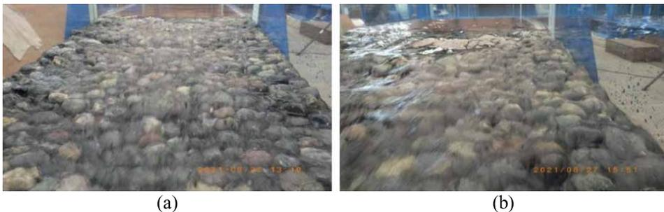
**Figure 7.** Flow conditions for a  $1/12.5$  downward slope and a  $1/11$  transverse slope. (a) Flow condition for Case 1. (b) Flow condition for Case 2.
