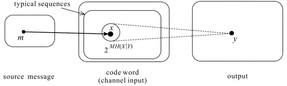
FIG. C.2. The original message  $m$  has a one-to-one correspondence with a code word  $x$ . There are  $2^{MH(X|Y)}$  possible inputs corresponding to an output of the channel. Only one of these  $2^{MH(X|Y)}$  code words (marked as a dot) should be the code word assigned to an original message.
