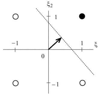
FIG. 7.9. Linearly separable task. The arrow is the vector  $\mathbf{J} = {}^t(J_1, J_2)$ .
