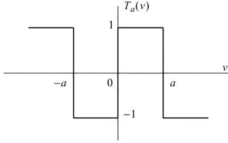
FIG. 8.3. Output  $T_a(v)$  of the reversed-wedge-type perceptron
