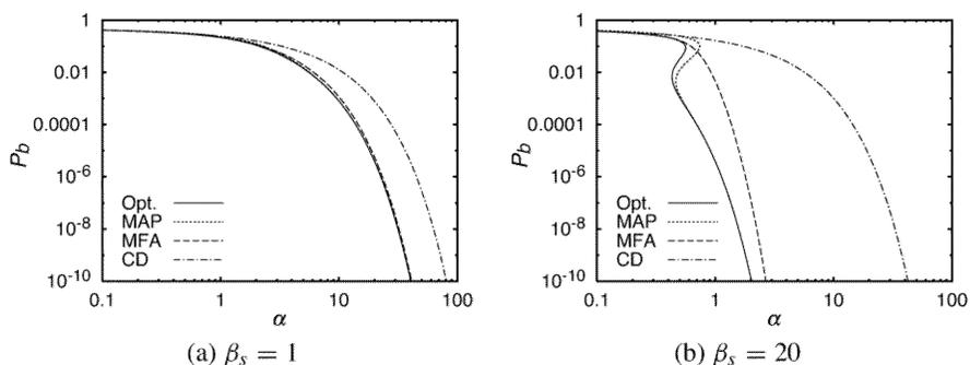
FIG. 5.14. Bit-error rate of the CDMA demodulators. The left one (a) is for the noise power  $\beta_s = 1$  and the right (b) is for  $\beta_s = 20$ . The symbols are: Opt. for the MPM, MFA for the mean-field demodulator with  $\beta = \beta_s$ , and CD for the conventional demodulator (T. Tanaka 2001; Copyright 2001 by the Massachusetts Institute of Technology).
