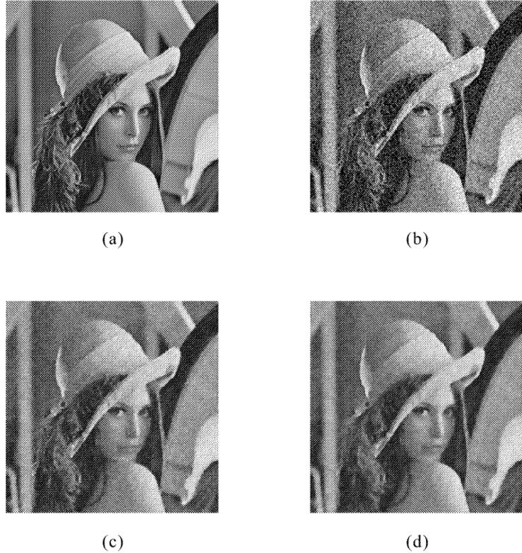
FIG. 6.4. Restoration of 256 grey-scale image by the Gaussian prior and edges (line process). Degradation was by Gaussian noise of vanishing mean and variance 900: (a) original image, (b) degraded images, (c) restored image by mean-field annealing, and (d) restored image by cluster variation method. Courtesy of Kazuyuki Tanaka (copyright 2001).
