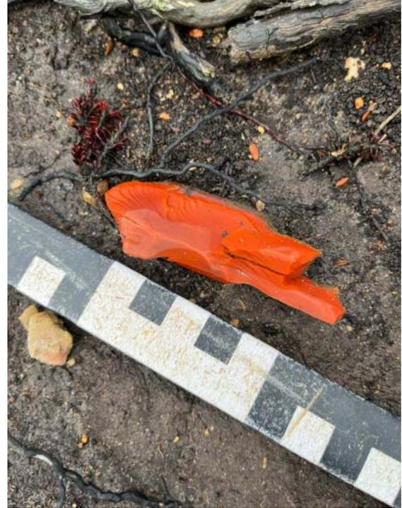
*Unburnt propellant in and around the wreckage
