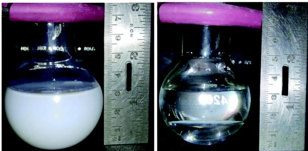
**Figure 1.** A digital image of a quartz reactor with a capacity of 70 mL (56 mm in diameter at the center) filled with 40 mL of solution and 25 mg of titania-based catalyst powder while it was spinning (left), and in static circumstances, using thin films produced with 1 mg of the same photocatalyst (right). Replicated from ref. [56].
