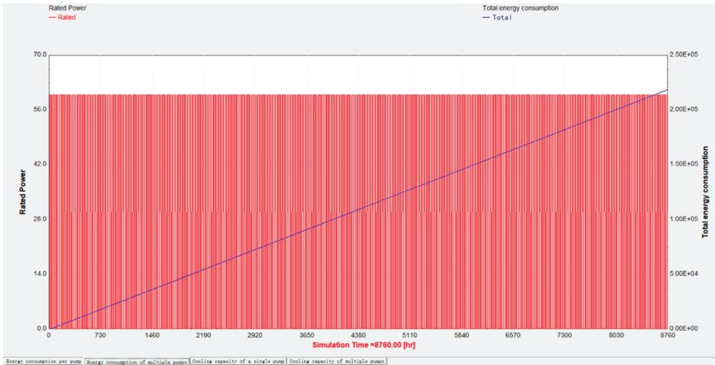
**Figure 11.** Scheme 2: annual cumulative energy consumption of several vacuum refrigeration pumps (unit: kWh).
