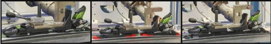
**Fig. 2** The bindings mounted directly to the ski without any additional ski plate (*left*), on the original ski plate (Tyrolia Raceplate RDX; *middle*) and on the new ski plate (Allflex plate; *right*)
