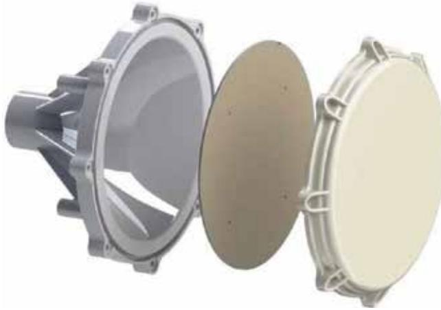
Figure 8. Perspective view of the complete transmitarray antenna [14].
