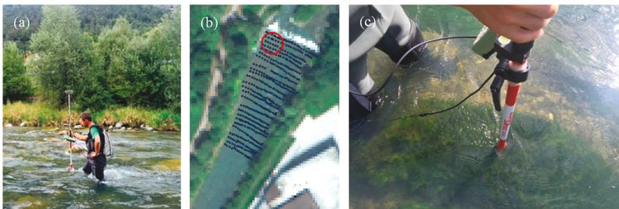
**Figure 14.** (a) Field observations to record water depths and SAV densities assisted by a precise RTK GPS, (b) cross-sectional measurement points of water-depths superimposed on the WV3 image, and (c) a sample of SAV in the Sarca River. The sampling area used for estimation of  $K_d$  is highlighted by a circle on the satellite image.
