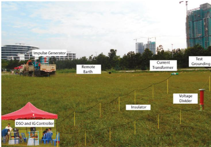
Figure 1. Equipment used for field measurements.
