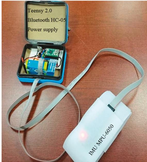
Figure 4. Portable foot attitude measuring device.
