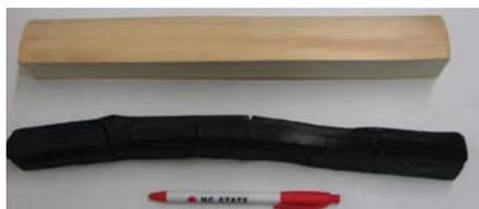
**Figure 4.** Comparison of oven-dried yellow poplar biomass (**top**) to the charcoal produced (**bottom**).
