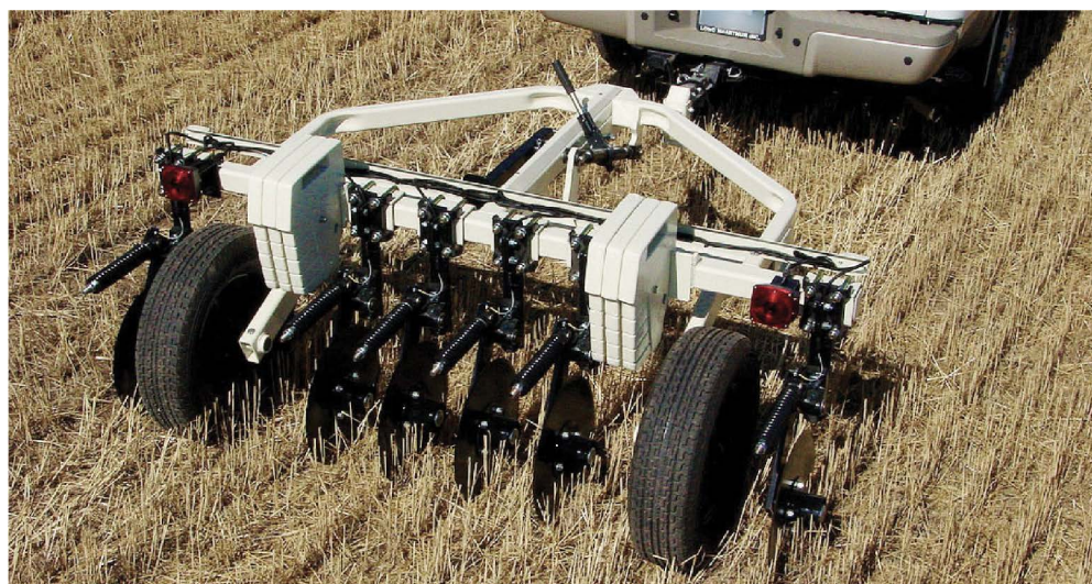
Fig. 59.3. Veris 3100 sensor cart used for collecting soil electrical conductivity data to make soil texture management zones for site-specific applications (Veristech.com). Photograph courtesy of Veristech.
