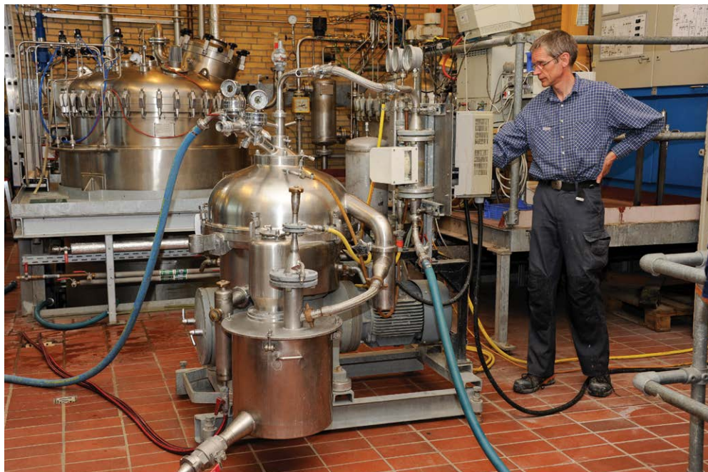
Fig. 62.3. Separator centrifuge for the concentration of liquid broth harvest of microorganisms. Photograph courtesy of e-Nema, Kiel, Germany.
