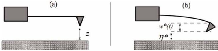
**Figure 2.** Scheme of the AFM system. (a) System in initial start and (b) intermittent.
