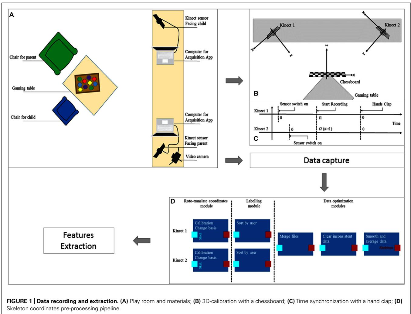
**FIGURE 1 | Data recording and extraction. (A)** Play room and materials; **(B)** 3D-calibration with a chessboard; **(C)** Time synchronization with a hand clap; **(D)** Skeleton coordinates pre-processing pipeline.
