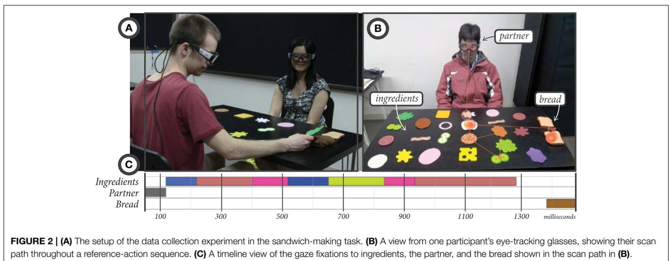
position accuracy of  $0.5^\circ$ . Each set of glasses contains a forward-facing high-definition camera that was used to record both audio and video (24 fps). The gaze trackers were time-synchronized with each other so that the gaze data from both participants could be correlated.
