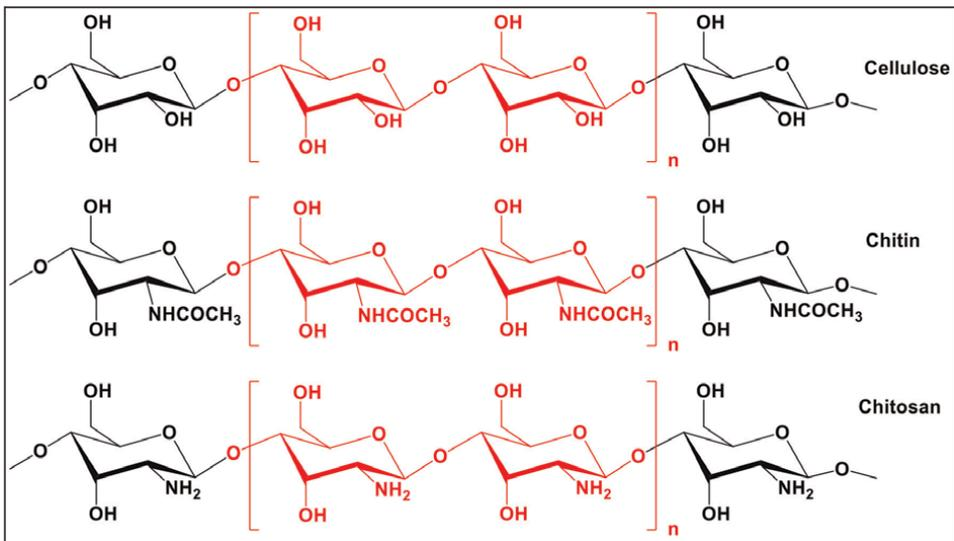
**Figure 1.** *Chitin, chitosan, and cellulose’s molecular structures [1].*
