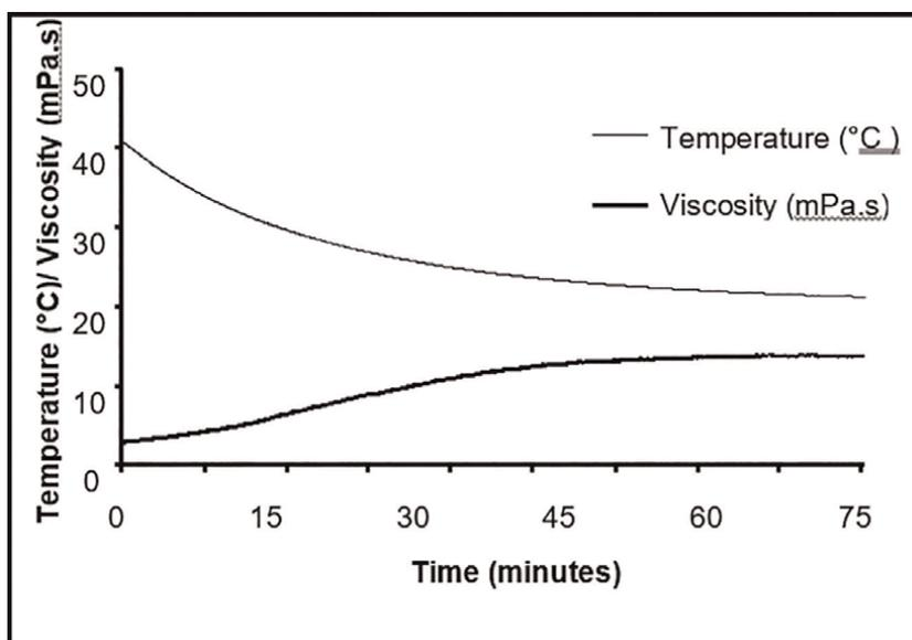
**Figure 4.** Temperature and apparent viscosity profile of WSCC in distilled water (5%, w/v) using SV-10 AND vibratory viscometer.
