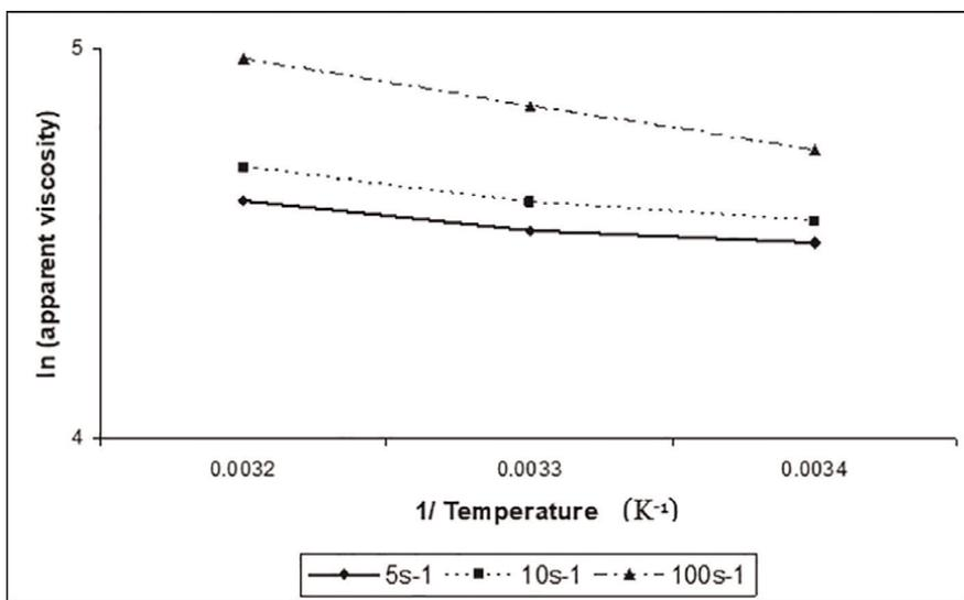
**Figure 3.** Arrhenius models of WSCC in distilled water (5%, w/v) at different shear rates and at different temperatures: Haake viscometer.
