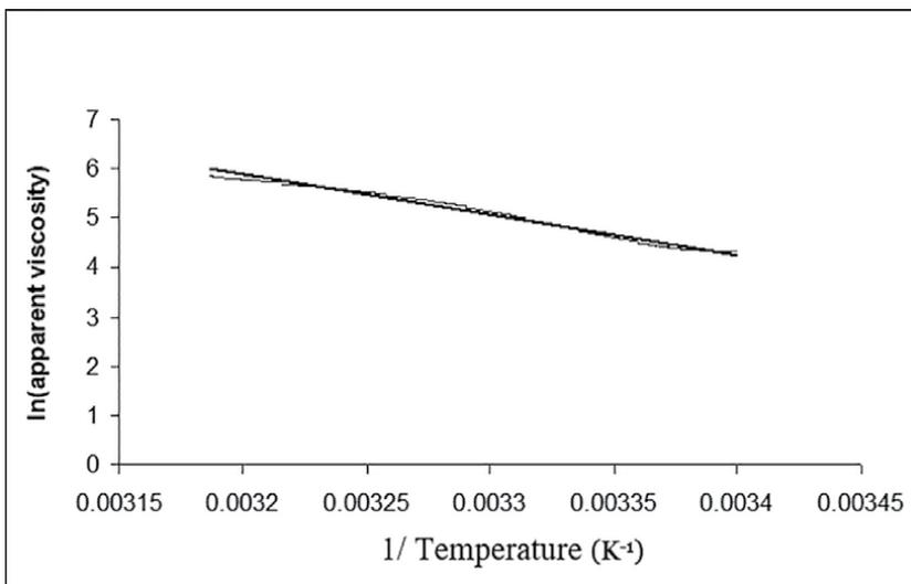
**Figure 5.** Arrhenius model of WSCC in distilled water (5%, w/v) at a single shear rate: SV-10 AND vibratory viscometer.
