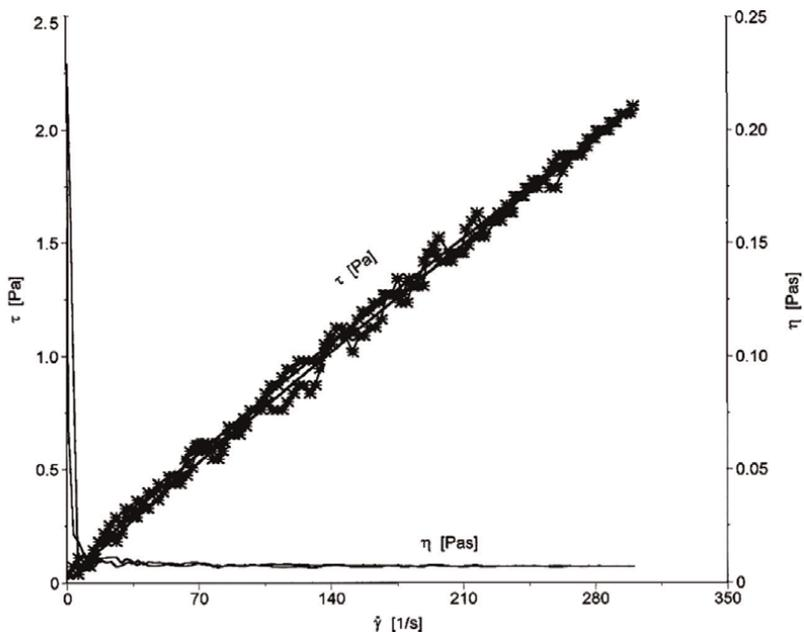
**Figure 2.** Flow curve obtained for WSCC dissolved in distilled water (5%, w/v) at 30°C using Haake viscometer.
