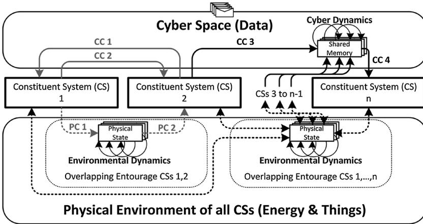
Fig. 4. Constituent Systems (CSs), Cyber Channels (CCs), and Physical Channels (PCs) at the cyber-physical interface layer
