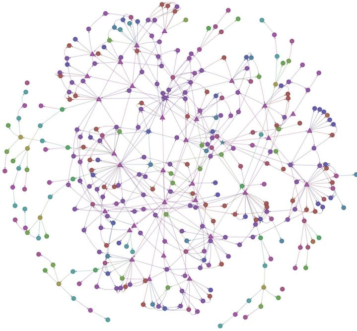
**Fig. 32.** The full SmartGrid model generated using the model query: “return true;” (i.e.: select all blocks). Here, the triangles represent systems, star represents the SoS and other blocks are represented by circles. The color of the blocks is the same as the one in the Blockly model.
