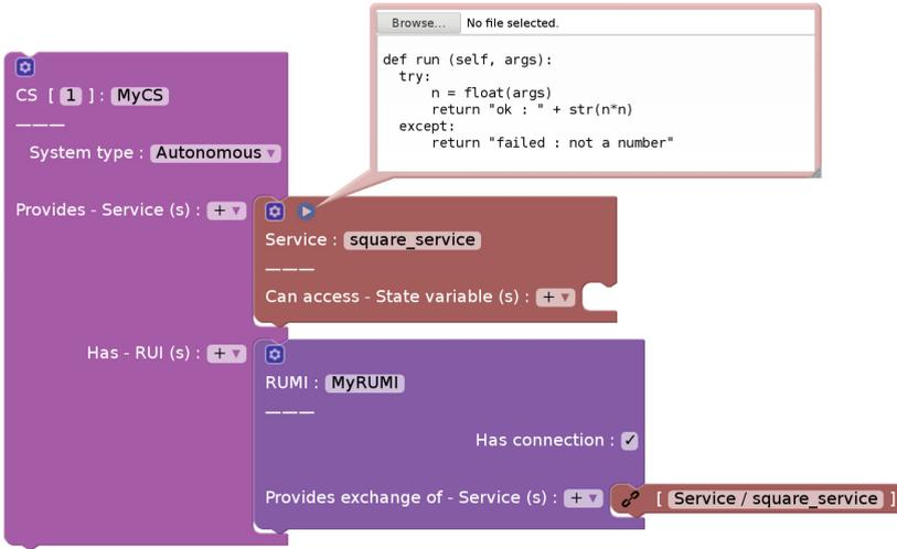
Fig. 28. Example of behaviour for a service
