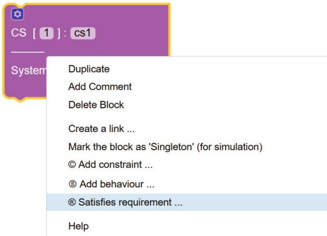
Fig. 19. Each block can satisfy a requirement (by providing the requirement ID it satisfies)
