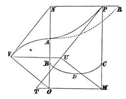
Let A be the lowest point of a uniform and perfectly flexible string hanging from two points under the action of gravity, Pany other point, AO the length of string whose weight is equal to the tension of the string at A.
