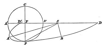
Let P be the position of the body at the instant the center of force is transferred from C, the center of the circle, to S, where SCP is an equilateral triangle.
