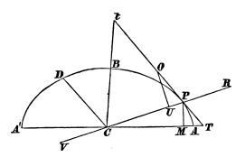
On *PC* produced, if necessary, take *PV* equal to four times the space through which a body must move from rest, under the action of the force at *P* continued constant, in order to acquire the given velocity *V*; so that  $V^{s} = 2\mu CP \cdot \frac{1}{4}PV$ .
