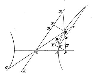
In the same manner as in these propositions, it can be shewn that the repulsive force tending from a focus, under the action of which the body describes the opposite branch of the hyperbola, varies inversely as the square of the distance.
