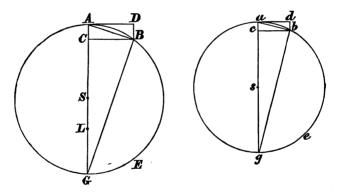
AD, ad tangents at A, a, ACSG, acsg diameters through A, a. Join AB, ab, and draw BC, bc perpendicular to AG, ag.
