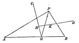
Let G be the center of gravity of two particles at A and B whose masses are in the ratio of  $\mu$  to  $\mu'$ , join PA, PB, PG.
