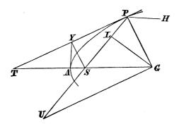
In this case, draw GL perpendicular to PS, and with S as focus, and 2PL as latus rectum describe a parabola, whose axis is in the direction SG.
