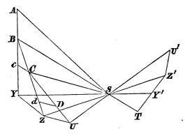
Draw SY, SZ, perpendicular to AB, BC; produce YS, ZS to Y', Z' making YS. SY' = ZS. SZ'.
