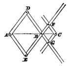
a point, which serves to fix the instrument to the drawing board, at A is a point, which is made to pass round the figure to be reduced or enlarged; at C is a hole for a pencil pressed down by a weight, and the pencil traces the similar figure, altered in dimensions in the ratio of BC : AB, or BF : AD.
