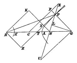
In this case, with S and H as foci, and HP-SP as transverse axis, describe a hyperbola, then PU is half the chord of curvature at P through S.
