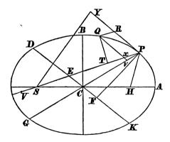
Let S be the focus to which the force tends, P the position of the body at any time, PCG, DCK conjugate diameters, Q a point near P, QT, PF perpendiculars on SP, DCK, from Q, P respectively, PR a tangent at P, QR parallel to SP, Qxvparallel to PR, meeting SP in x, and PC in v, and let SP, DCK intersect in E.
