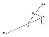
weights equal to those of the rods being placed at A, B, C; let AM be vertical and BM horizontal, and produce CB to meet AM in D, draw DN perpendicular to AB.
