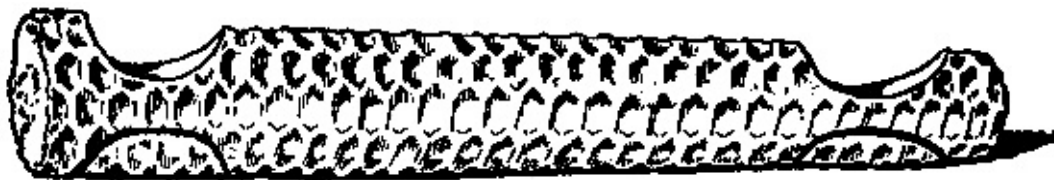
Fig.198 - Corn-cob log for pioneer log cabin with notches cut and marked.
